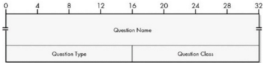
Figure 57-3. DNS message Question section format
