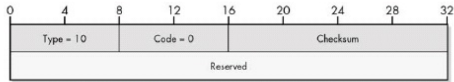
Figure 33-4. ICMPv4 Router Solicitation Message format
